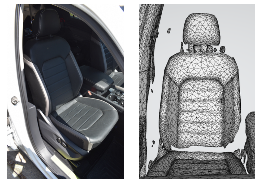
Figure 1. 3D scan of the vehicle seat (Patient 1).
